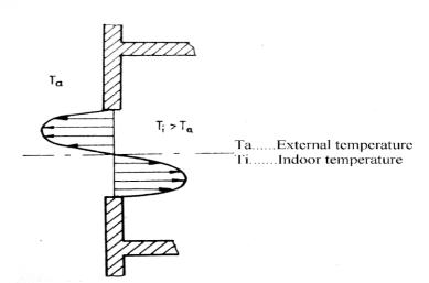
Figure 4.17.: Velocity profile of an open window
