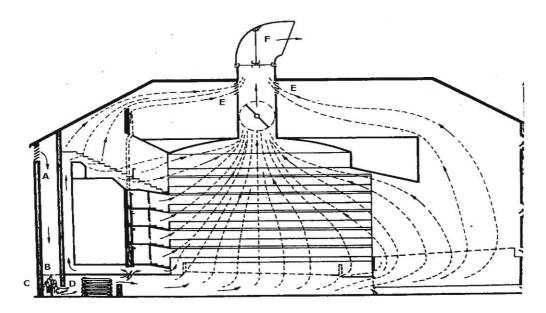
Figure 4.1.: Ventilation of a theatre after Reid (1844) [21] A – Supply air; B - air filtration; C – humidifying; D – heating; E – exhaust air; F – turn able fan outlet
