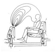
Figure 4.10.: Local restricted mixture of supply- and used-air
