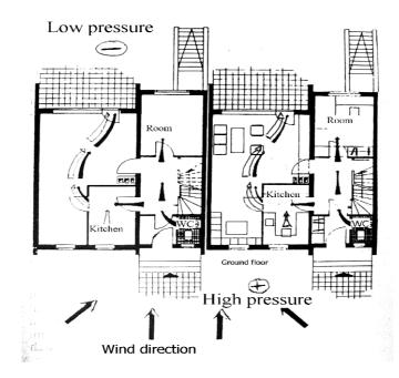
Figure 4.3.: Odour distribution due to wind. [33]
