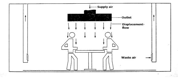
Figure 4.14.: Displacement aeration at a working station
