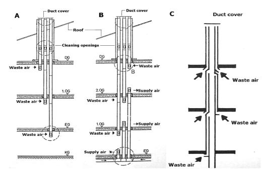
Figure 4.6.: Various schematic methods of duct ventilation.
