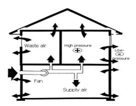
Figure 4.8.: Schema of a Supply-only ventilation system.[34]
