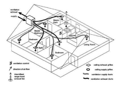
Figure 4.9.: Balanced ventilation schematic.[35]
