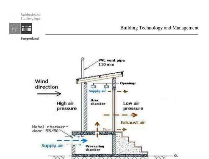
Figure 6.15.: Air flow scheme – section A – A. Kisoro, Mgahinga office.
