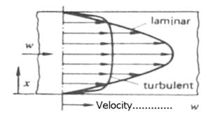
Figure 4.18.: Laminar and Turbulent flow.
