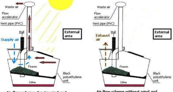
Air flow scheme due to wind and solar radiation.
