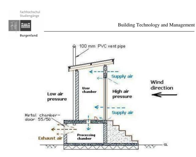
Figure 6.12.: Air flow scheme – section A - A. Kisoro, Karumena Village.
