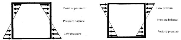
Figure 4.2.: Air flow due to temperature (pressure) differences.
