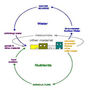
Figure 3.3.: Circular flow in an EcoSan system. [18]
