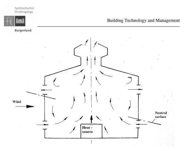
Figure 4.16.: Flow image of a free ventilation [36]
