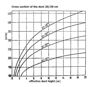
Figure 4.5.: Waste air stream [m<sup>3</sup>/h] due to temperature difference and effective duct height. [23]
