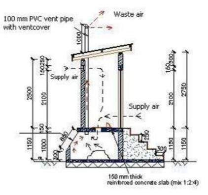
Figure 6.1.: Cross section of a double vault dry toilet – Type Kabale.
