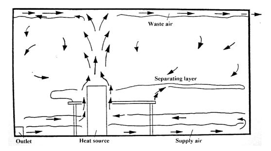
Figure 4.15.: Flow illustration of a source aeration
