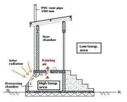
Figure 6.18.: Air flow scheme – section A – A. Kabale, Nyabiconi Rutenga.
