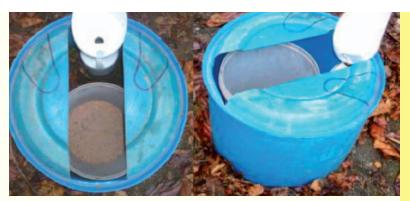
Figure 1: Simple, portable UDDT made from a discarded plastic barrel, a bucket, and two plastic bottles. Note the marks for placement of the feet.
