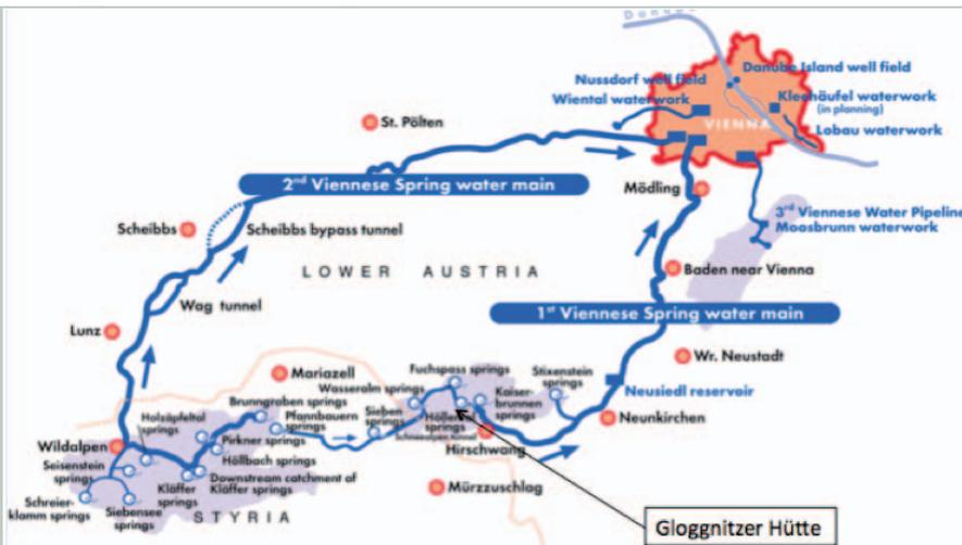
Figure 1: Overview on the catchment of Vienna Waterworks and the site of the 'Gloggnitzer Huette' (Source: www.wasserwerk.at). Shaded areas mark zones of water protection. Blue lines are the water supply mains of Vienna.
