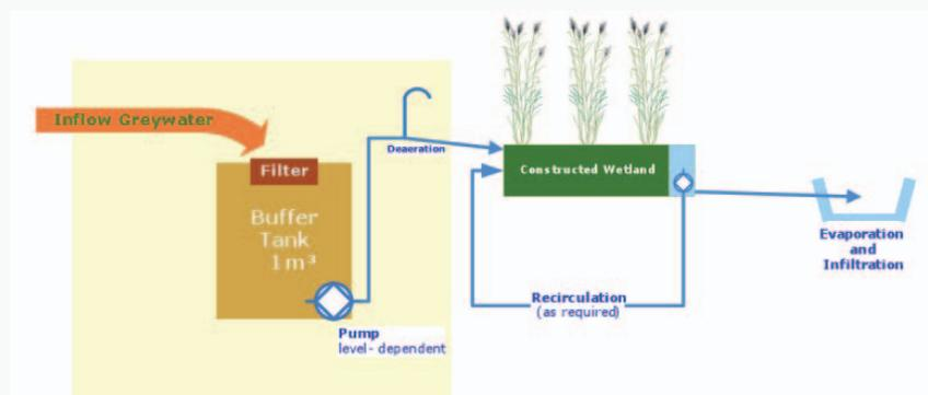
Figure 4: Scheme of the greywater and urine treatment.
