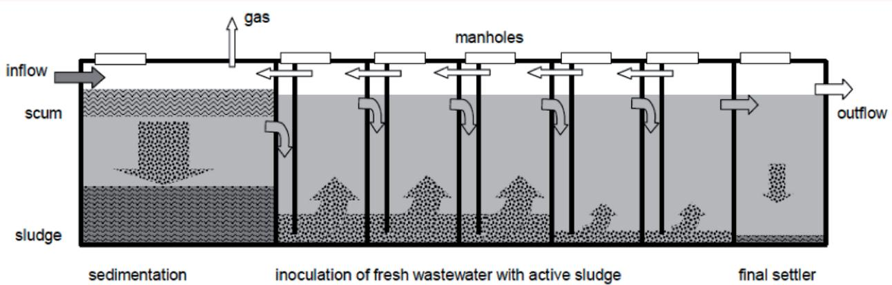
Figure 4: Wastewater flow through an ABR TED BORDA 2006
