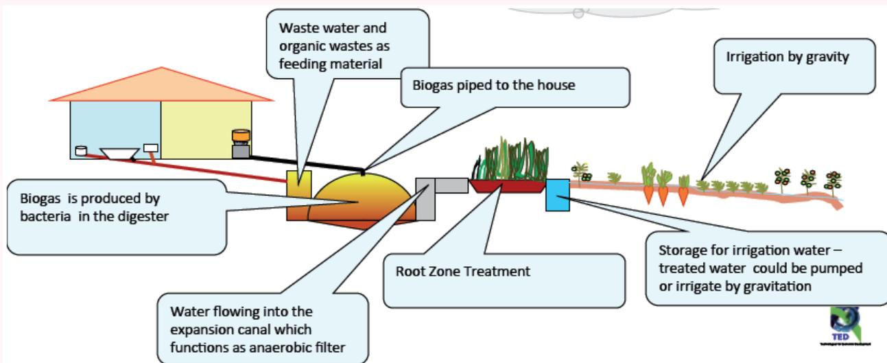
**Figure 2: Original TED design for biogas sanitation**
