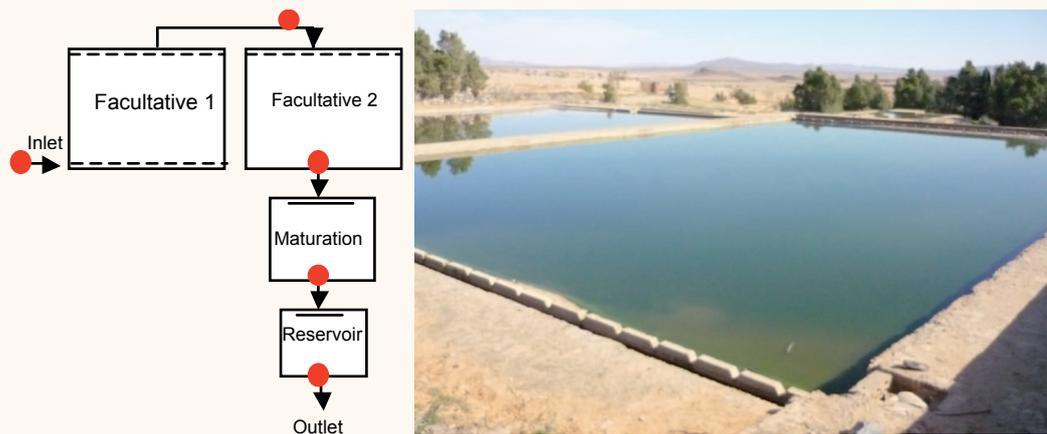
Figure 4. Flow diagram of Hammam Foukani’s WSP, sampling points and view of the facultative ponds
