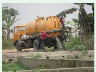
Figure 8: Opening a sluice valve of a tanker at "Bois des singes"
