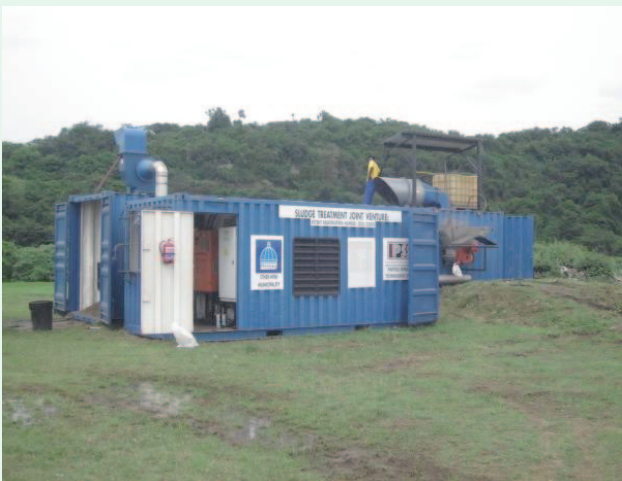
Figure 2 – The LaDePa machine assembled in a container.
