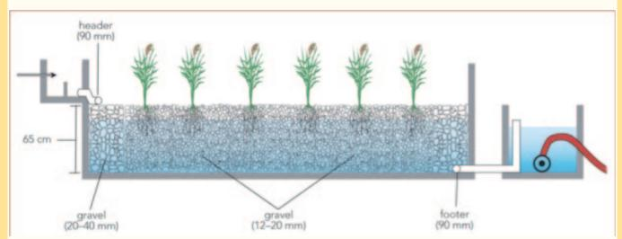
Figure 4: Secondary HF Wetland Cross Sectional View
