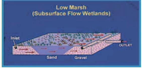
Figure 1: Schematic sketch of a CW bed with HSSF
