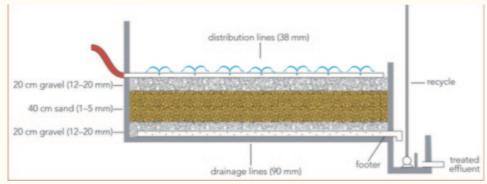
Figure 6: Tertiary VF Sand Filter Cross Sectional View
