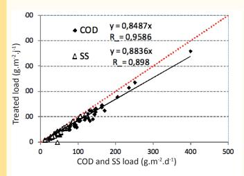
Figure 8: Treated COD and SS on the first stage for 0.1 < HL <1.57 m/d.
