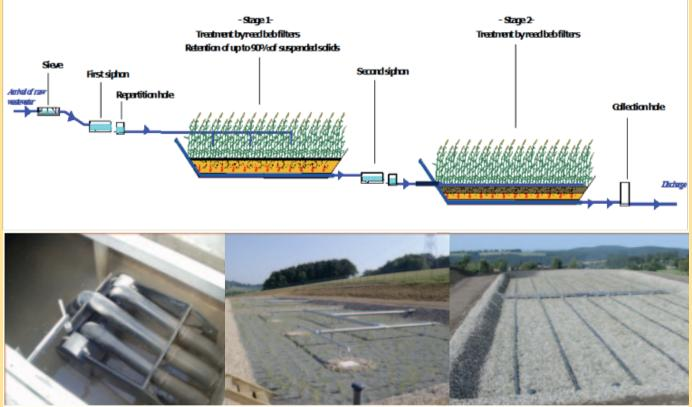
Figure 3: VF CW configuration with siphon
