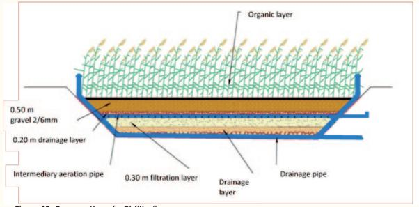
Figure 13: Cross section of a Bi-filtre®
