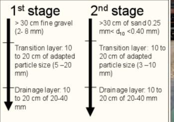
Figure 4: Particle size profiles (IRSTEA guidelines)
