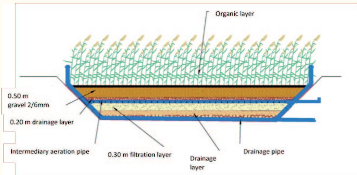
**Figure 13: Cross section of a Bi-filtre<sup>®</sup>**
