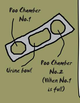
A UDDt source separates the pee & poo (along with the wash water), which can then be treated separately before reuse. The faeces are sanitised by containing and desiccating them in the tanks below. The urine can be stored and used on dilution or percolated directly along with the wash water.
