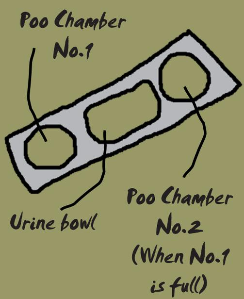
A UDDt source separates the pee & poo (along with the wash water), which can then be treated separately before reuse. The faeces are sanitised by containing and desiccating them in the tanks below. The urine can be stored and used on dilution or percolated directly along with the wash water.
