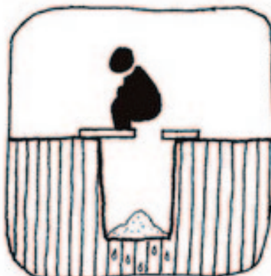
A soak pit is where the ground acts like a sieve
