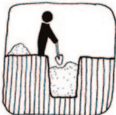
poo collects in the pit and must be removed
