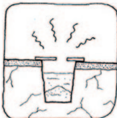
Soak pits don't work with hard, rocky ground
