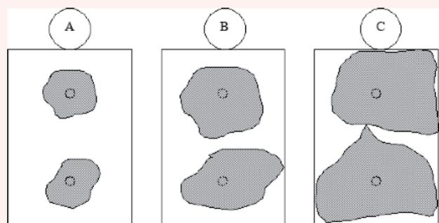
**Figure 3:** Plan view of surface layer area evolution in a bed of Glandieu during 12 day assay. Circles represent feeding points, from no surface layer at day 0 to (a) day 2; (b) day 4; and (c) day 12. Adapted from Chazarenc and Merlin (2005).
