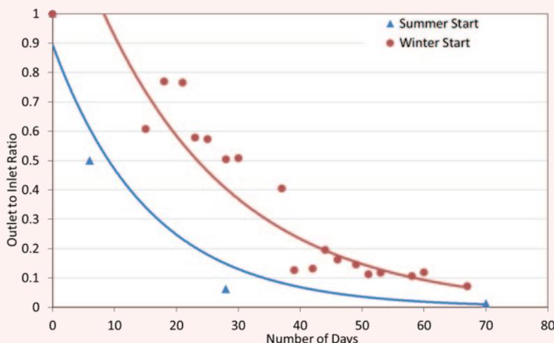
**Figure 4: Outlet to inlet ammonium concentration ratios during the start-up phase for two aerated wetland systems in the UK (ARM, Ltd).**
