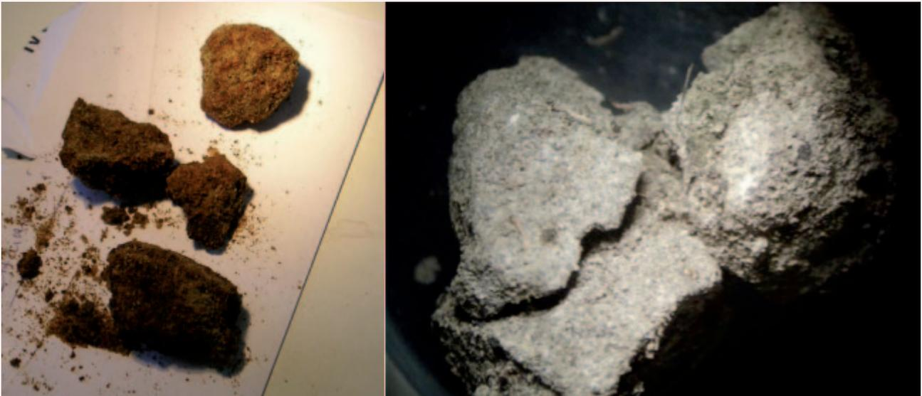
**Figure 8: Chemical precipitation within wetland media leading to clogging (a) sand and iron clusters from a VF wetland, (b) media cementation from a steel slag pilot wetland in the UK. Images courtesy of (a) D. Van Oirschot and (b) Flint Walters.**
