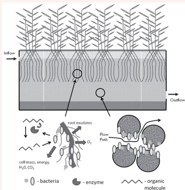
**Figure 1: Simplified depiction of microbial community interactions with bed media, plant roots, and organic wastewater components in a horizontal subsurface flow treatment wetland system. (Diagram not to scale)**
