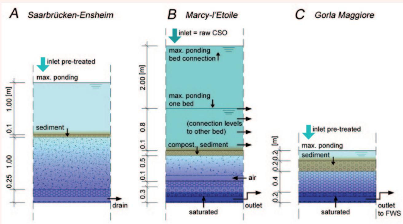
Figure 2: Simplified cross-sections of CSO-CWs in (A) Germany, (B) France and (C) Italy (Meyer et al., 2013)
