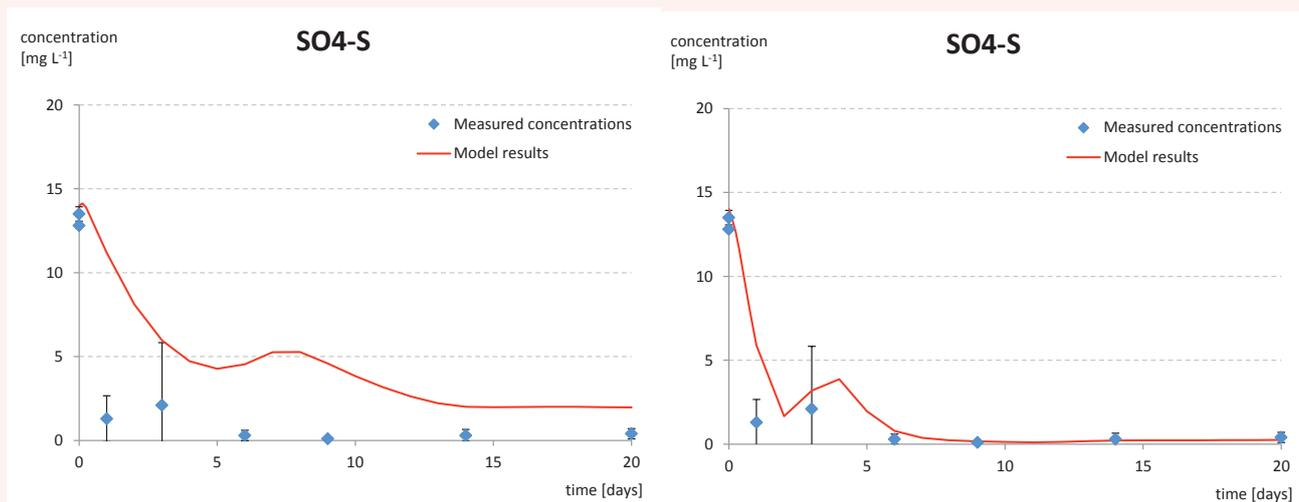
**Figure 2: Measured and simulated sulphate concentrations for a batch-fed column at 24°C planted with Carex (left: using the standard parameter set of the biokinetic model; right: after adaptation of inhibition and half-saturation coefficients to allow anaerobic, anoxic and aerobic processes to occur in parallel; Pálffy, 2013)**
