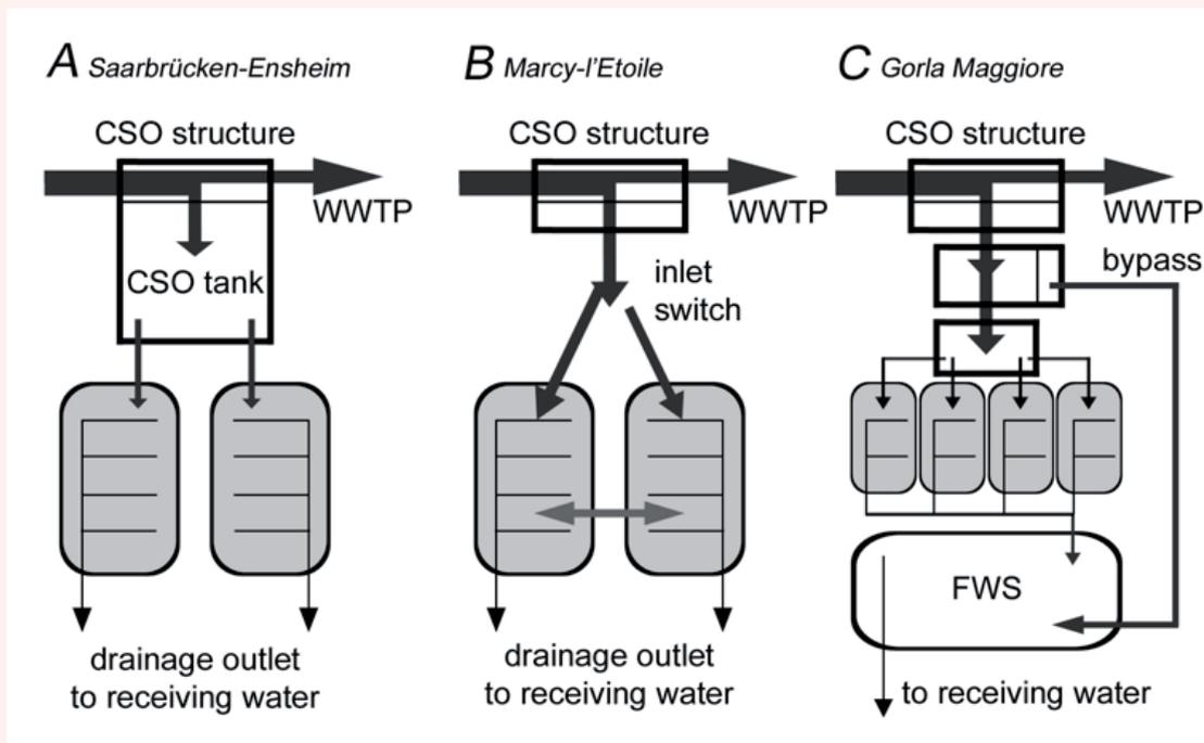
Figure 1: Simplified system sketch for (A) RSFs in Germany, and CSO-CWs in (B) France and (C) Italy (Meyer et al., 2013)
