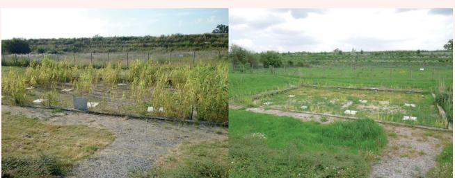
Figure 4c: Hauterive second stage French system reed bed, July 2012, showing poor health and disappearance of reeds creating significant reed-free areas (courtesy Joëlle Paing) Figure 4d: Hauterive second stage French system reed bed, May 2013, almost complete disappearance of reeds within three years of first yellowing, with replacement by "weeds" (courtesy Joëlle Paing)
