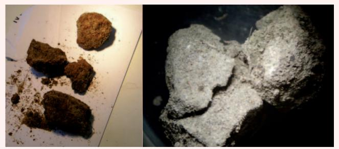
Figure 8: Chemical precipitation within wetland media leading to clogging (a) sand and iron clusters from a VF wetland, (b) media cementation from a steel slag pilot wetland in the UK. Images courtesy of (a) D. Van Oirschot and (b) Flint Walters.
