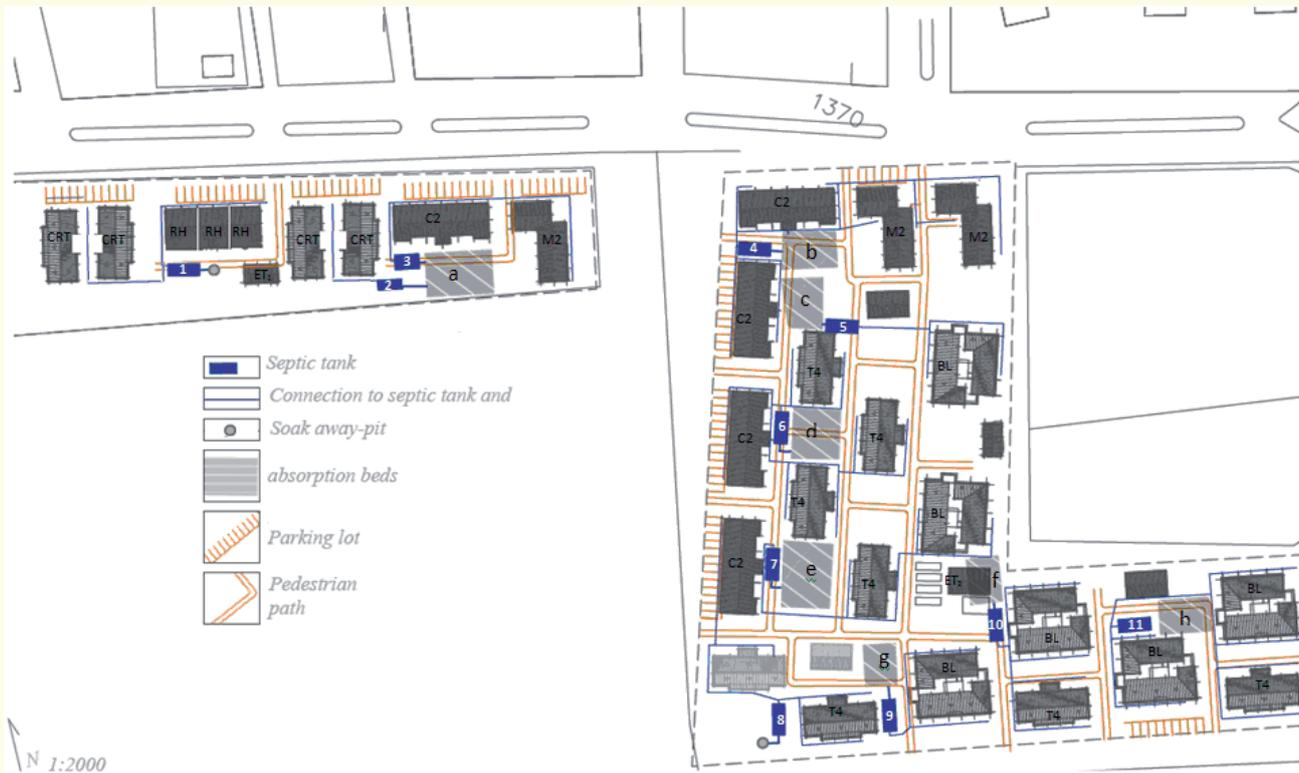
**Figure 2: Site plan of the Bekele Mola condominium house area including supply and disposal structures (Augustsen and Hauso, 2012).**
