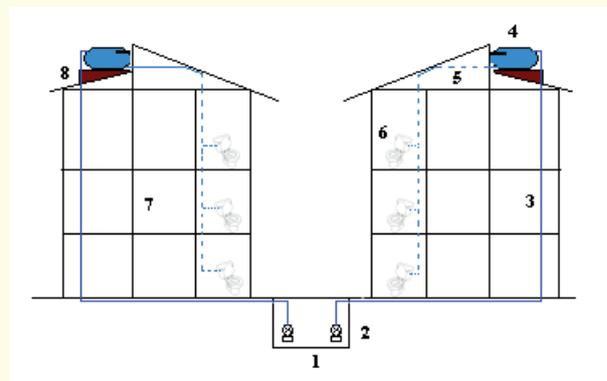
Figure 4: (1) Underground storage tank, (2) submersible pumps, (3) pipe connections, (4) elevated storage tank 2 m3, (5) pipe connection, (6) flush toilet reservoir, (7) multi-storey buildings, (8) support for elevated tank.
