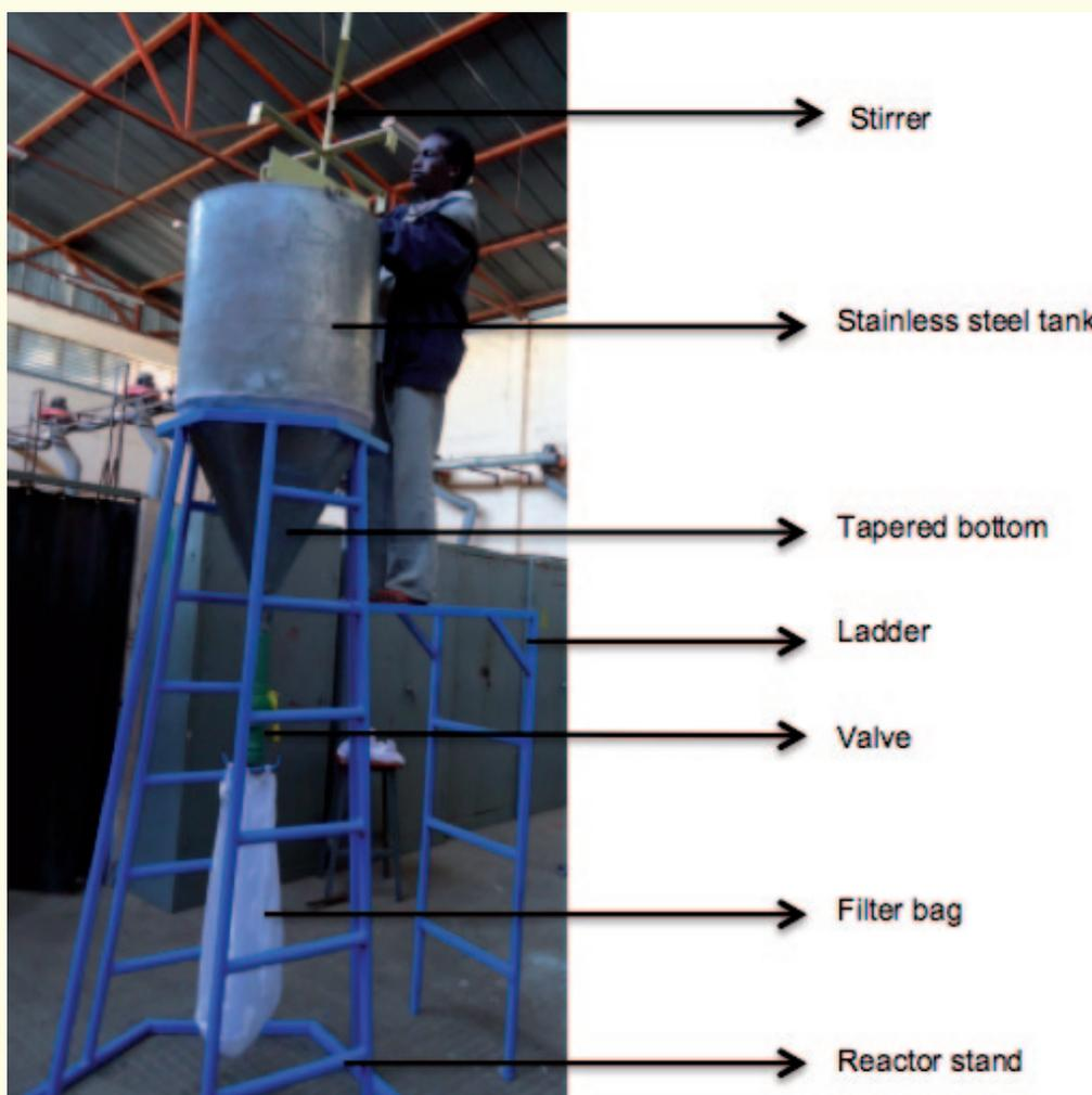
Figure 1: Struvite precipitation reactor
