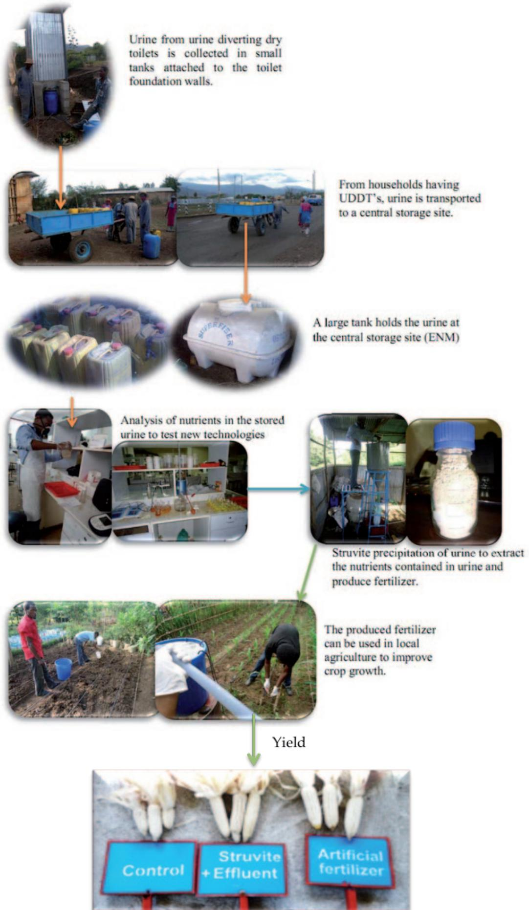
Figure 2: Overall process of nutrient recovery from source-separated urine in Arba Minch
