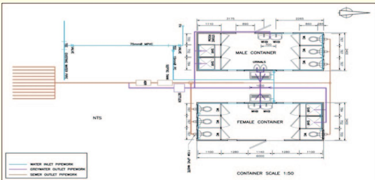
Figure 5: Process Flow Diagram of a typical CAB system
