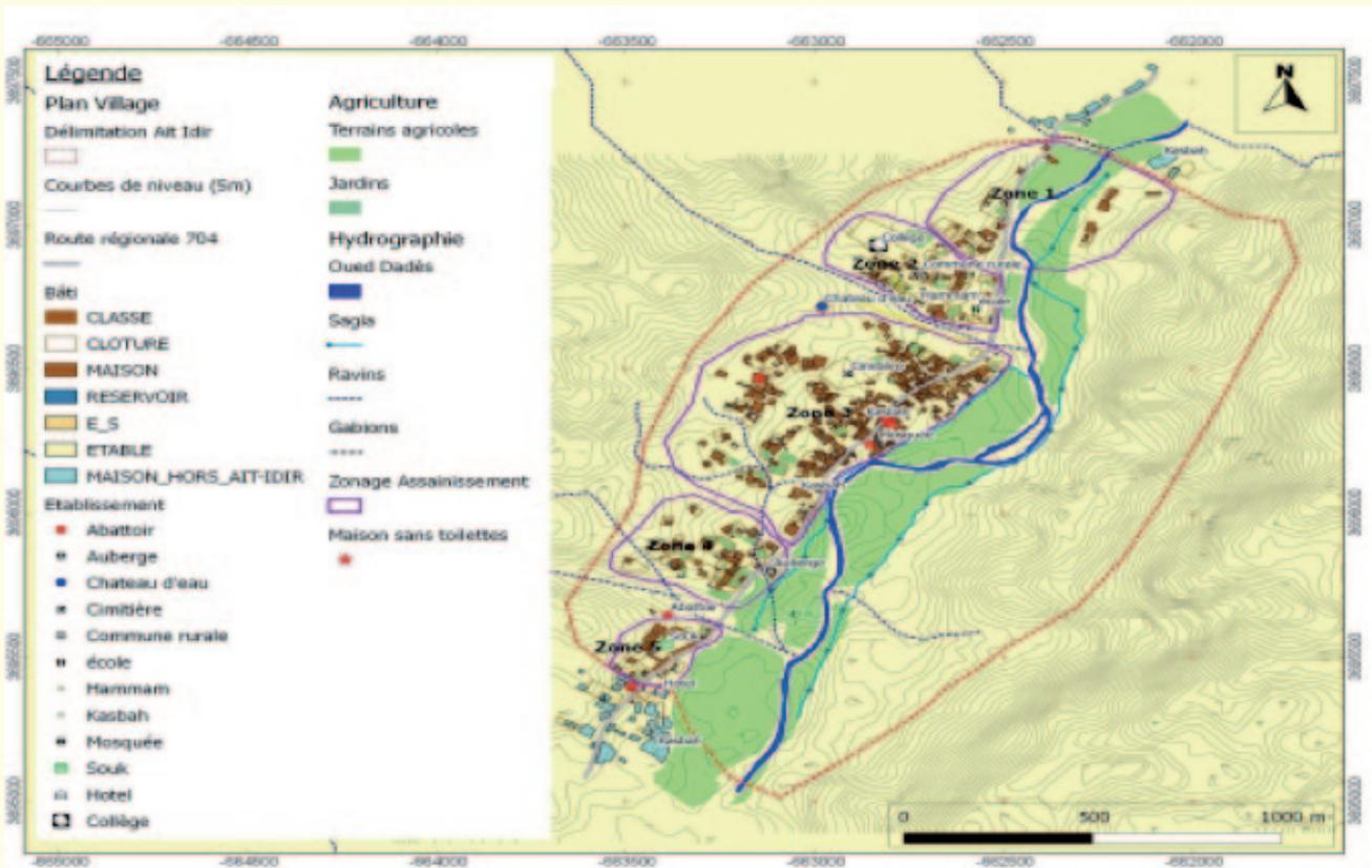
Figure 3: The green areas are potentially available for wastewater treatment plant in Ait Idir.
