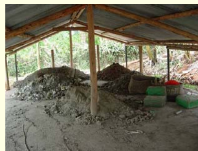
Figure 4: Drying and storage area for faecal material.
