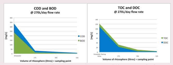
Figure 2: Cleaning performance of the Vertical Ecosystem for COD and BOD (left) and TOC and DOC (right).
