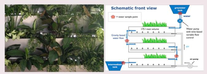
Figure 1: Vertical Ecosystem - laboratory test unit (left) schematic front view of the Vertical Ecosystem (right)
