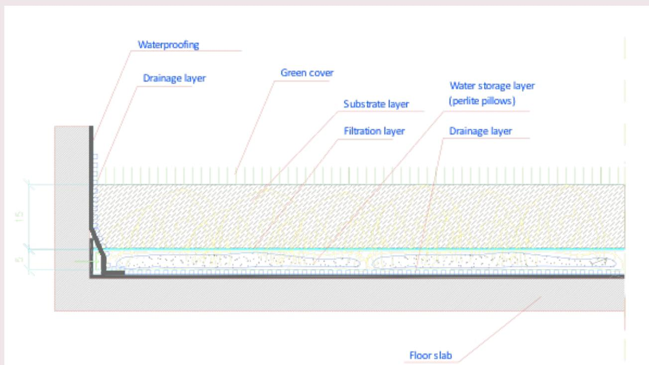
Figure 4: Green roof filling layers
