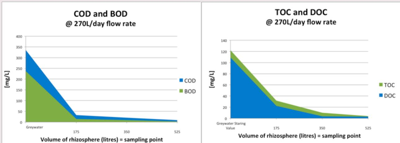
Figure 2: Cleaning performance of the Vertical Ecosystem for COD and BOD (left) and TOC and DOC (right).
