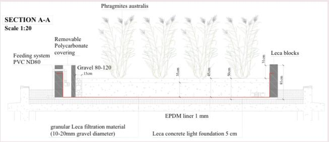
Figure 1. Section of the roof wetland designed for Grumeti Community of Serengeti, Tanzania
