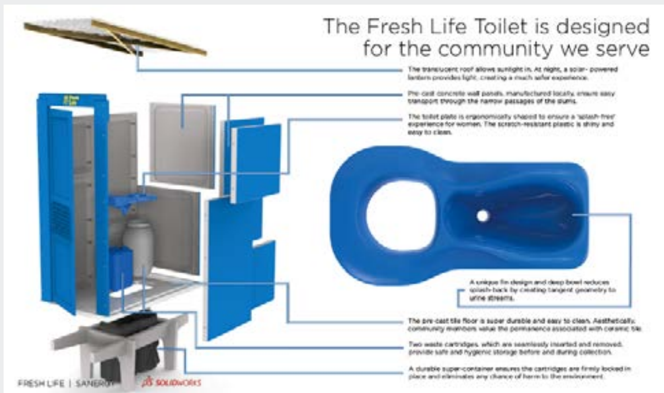
Figure 1: The Fresh Life Toilet has a unique urine-diverting squat plate and cartridge collection system.
