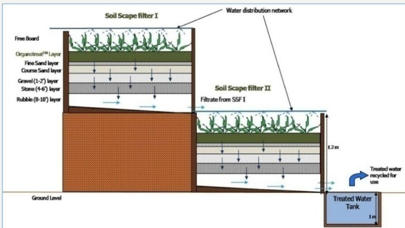
Figure 4 - Cross section of soil scape filter units
