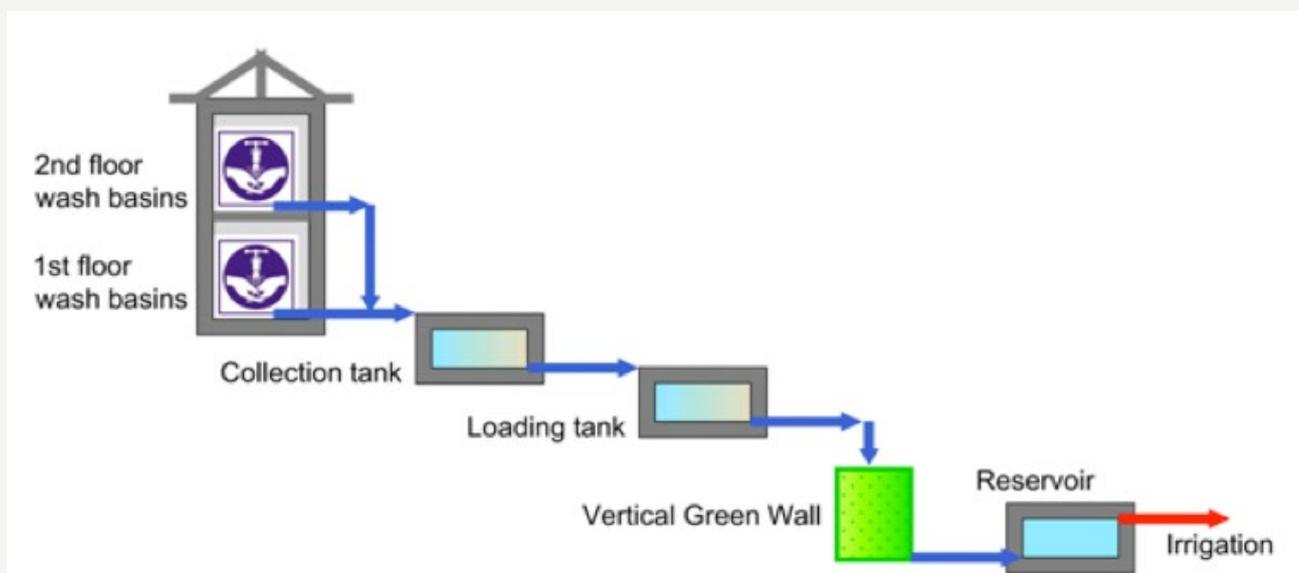
**Figure 1: Sketch of the greywater treatment unit**
