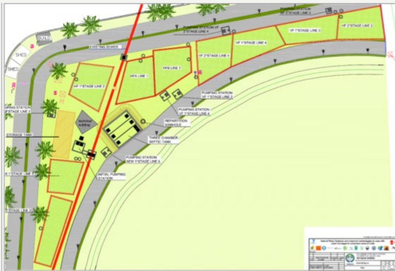
Figure 1: Schematic of the treatment system (source: Iridra and Kreta, 2014)
