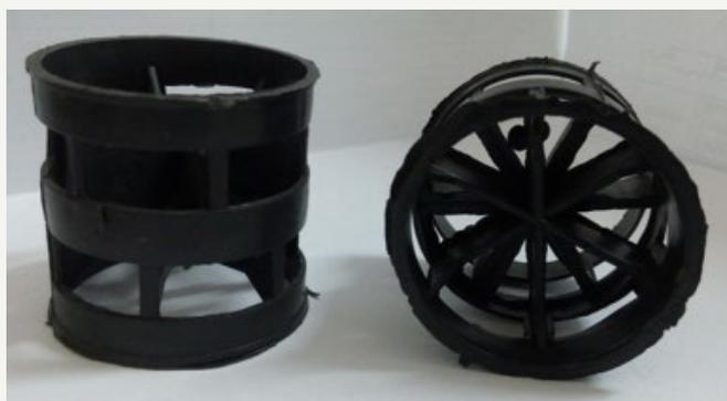
**Figure 2: Anaerobic filter media (Pall rings) made of PP/HDPE featuring high specific surface area 150 – 200 m<sup>2</sup>/m<sup>3</sup>**
