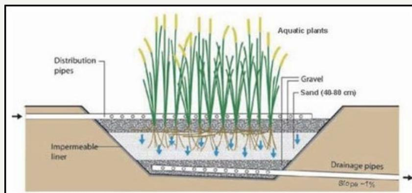
Figure 2: Schematic diagram of vertical flow constructed wetland
