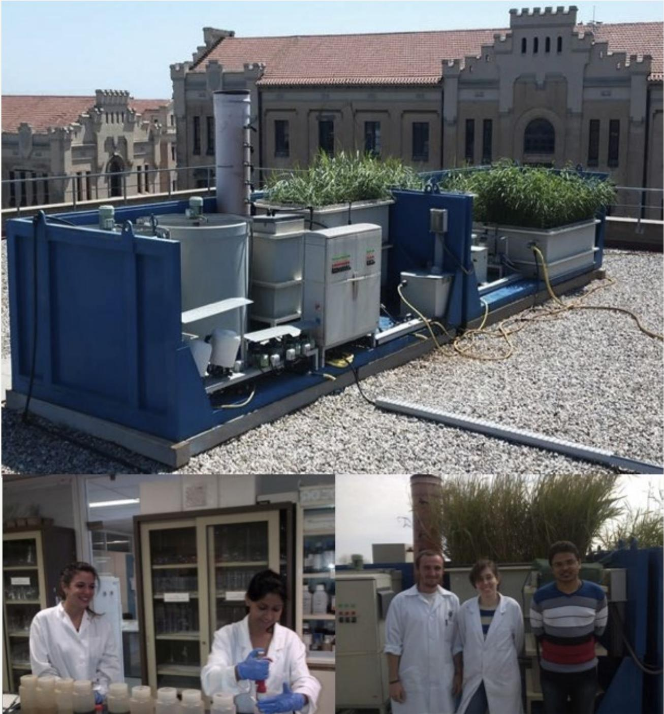
**Figure 2. View of the three-stage hybrid constructed wetland system and some of the students involved in the monitoring of the system**
