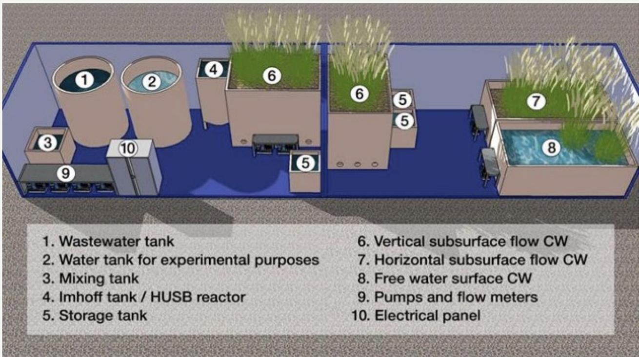
Figure 1. Layout of the pilot three-stage hybrid constructed wetland system (Ávila et al., 2013)
