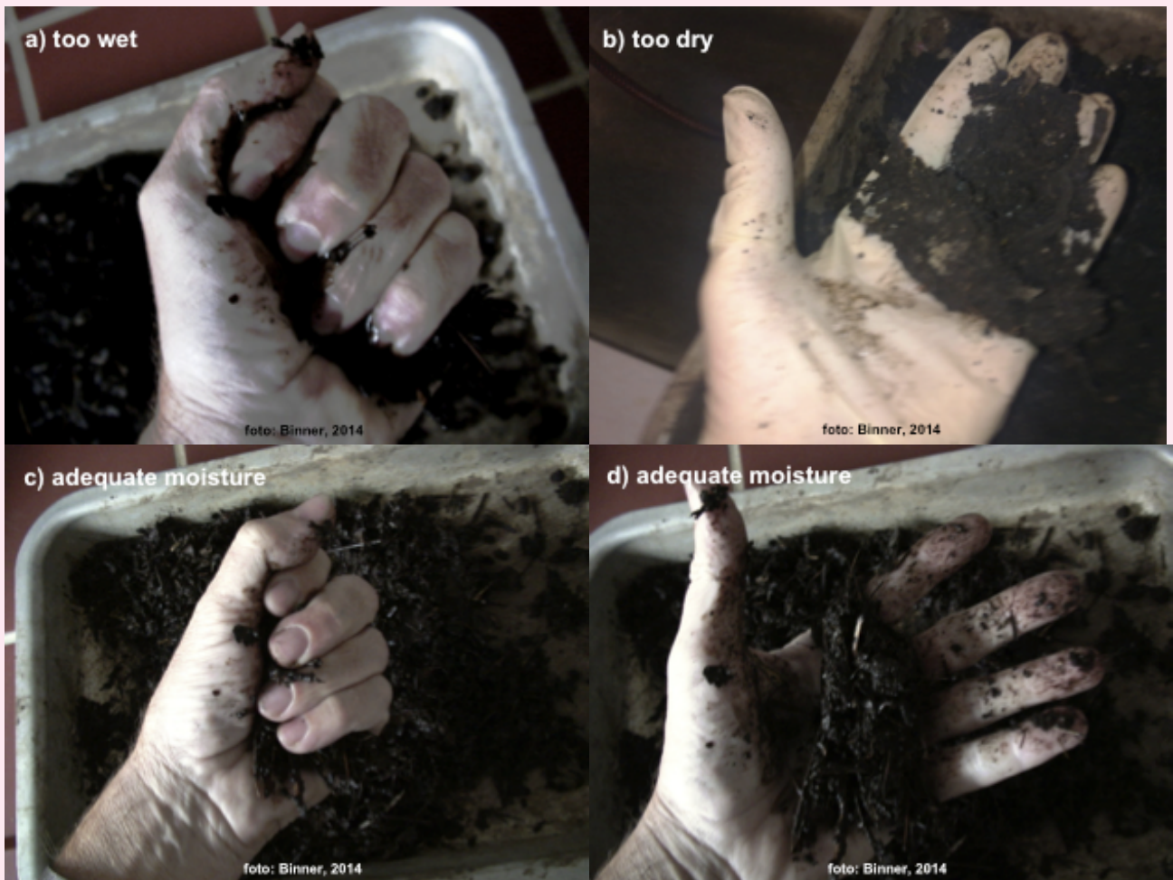
Figure 9. Fist test for evaluation of moisture content during composting a) too wet b) too dry c) and d) adequate moisture.
