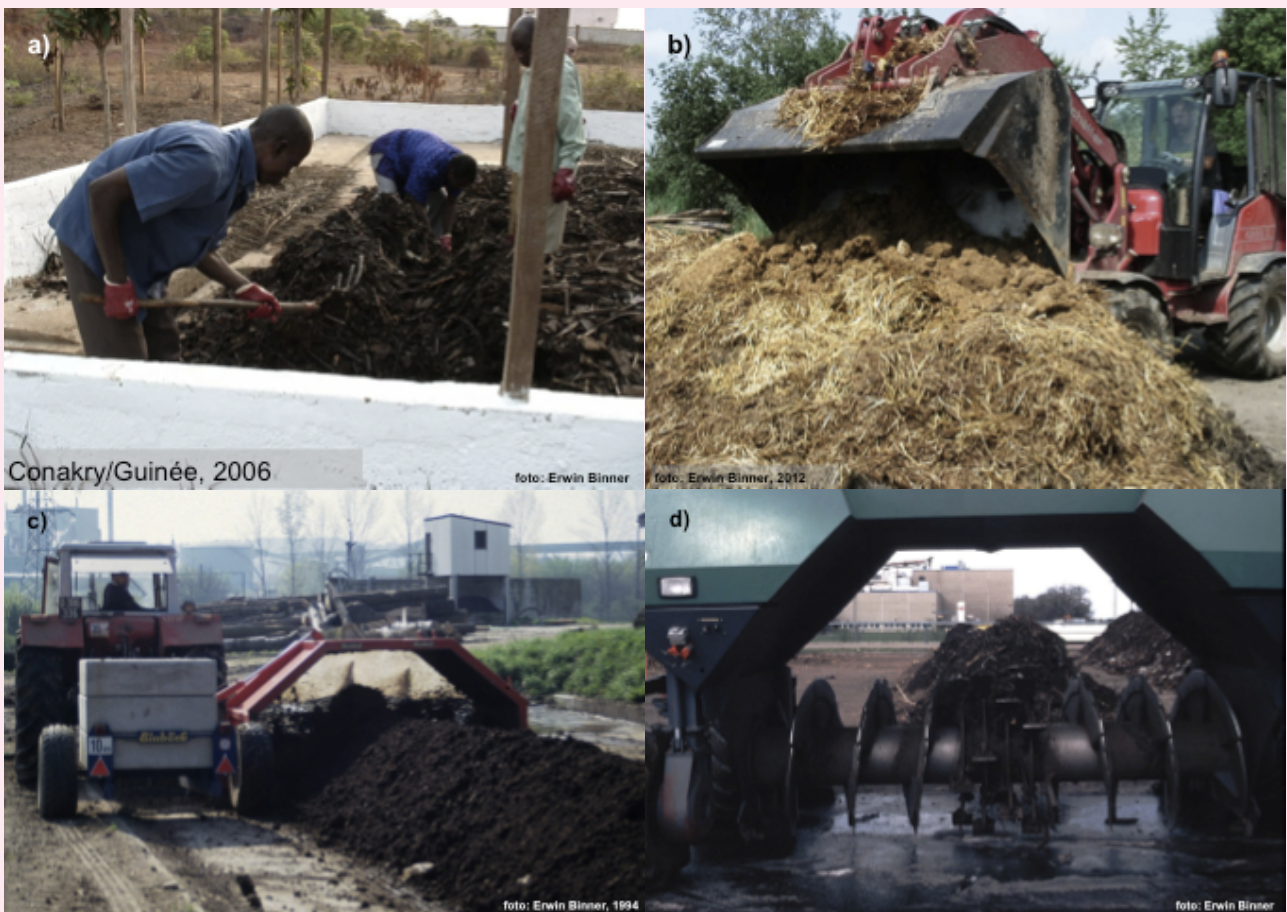
Figure 12. Turning of windrows a) manual b) front-end loader c) turning machine d) detail of a self-powered turning machine.
