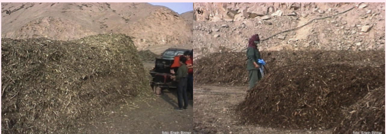
Figure 8. a) Windrow, too high related to feedstock properties b) windrow according to feedstock properties.
