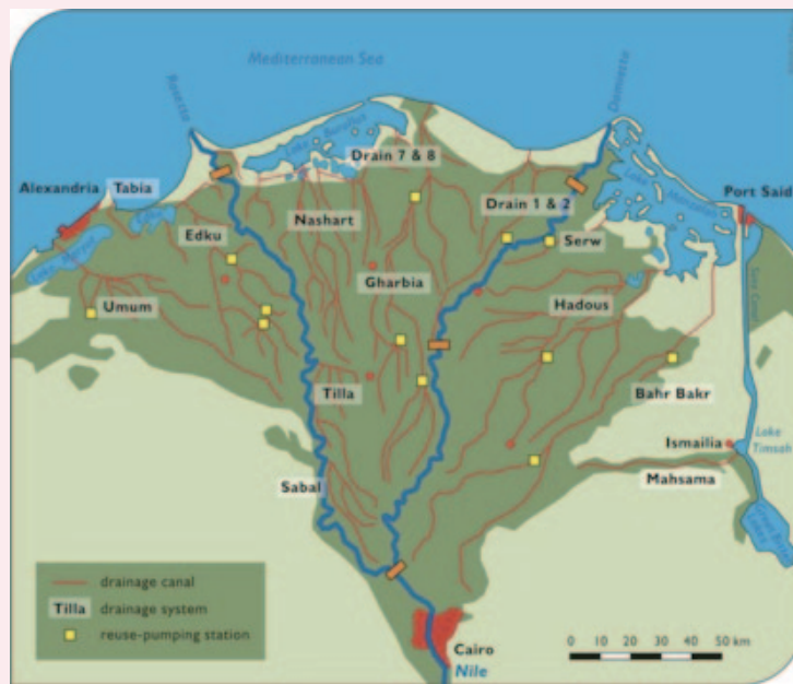
Figure 3: Main drainage Canal in the Delta region, Egypt (Abdel-Wahaab, 2003).
